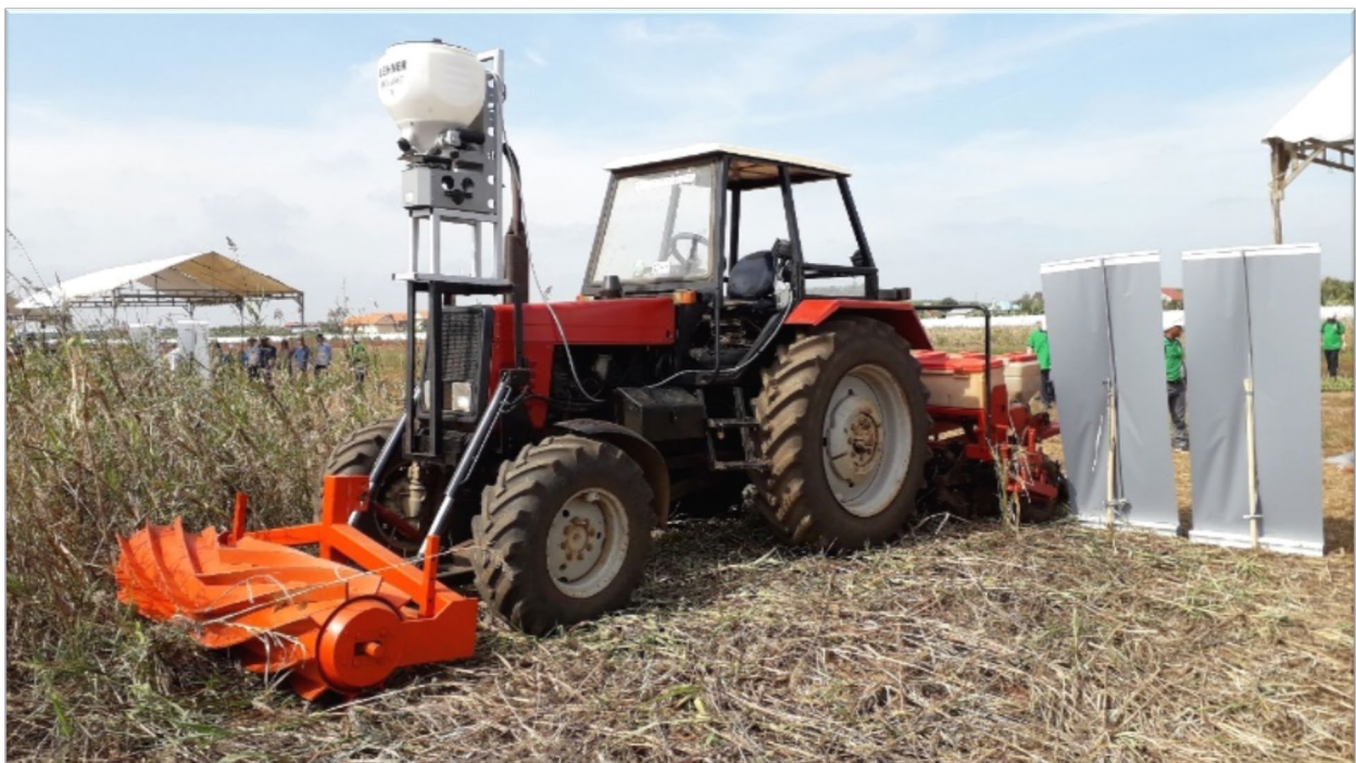
Figure 3: Demonstration of roller crimper, no-till planter and seed broadcaster by the Department of Agricultural Land Resources Management and the Conservation Agriculture Service Center
