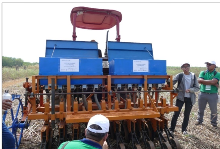
Figure 1: Demonstration of rice no-till seeder developed by the Department of Agricultural Engineering through the project Appropriate-scale Mechanization Consortium (ASMC)
